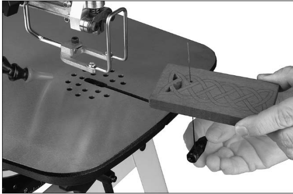
Figure 16: installing blade with workpiece
